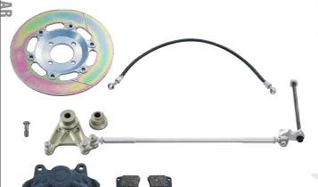
JB-POWER Rear Floating Brake Kit [Cast Iron Disc φ250, CP2696 Caliper, Brake Pads, Caliper Bracket [Collar included], Torque Rod, Torque Rod Anker, Stainless Mesh Brake Hose, Stainless Fitting, Banjo Bolt]
